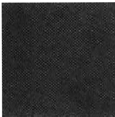
Figure 4.41 Cotton is treated with pre-mordanting process using the ferrous mordant before dyeing the solution from eucalyptus leaves
