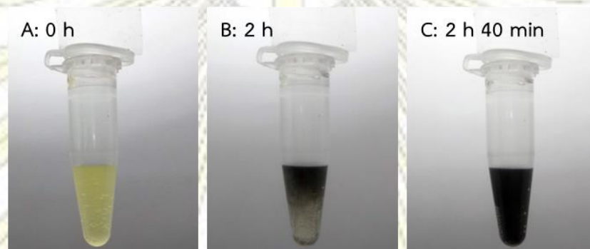
Figure 3.2 Color of \text{H}_2\text{PtCl}_6 and HCOONa mixture at A: 0 h, B: 2 h, and C: 2 h 40 min
