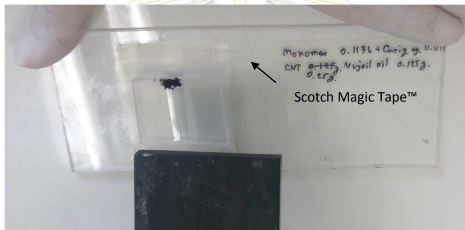
Figure 3.6 The electrode paste was filled into the channels on a PDMS plate.
