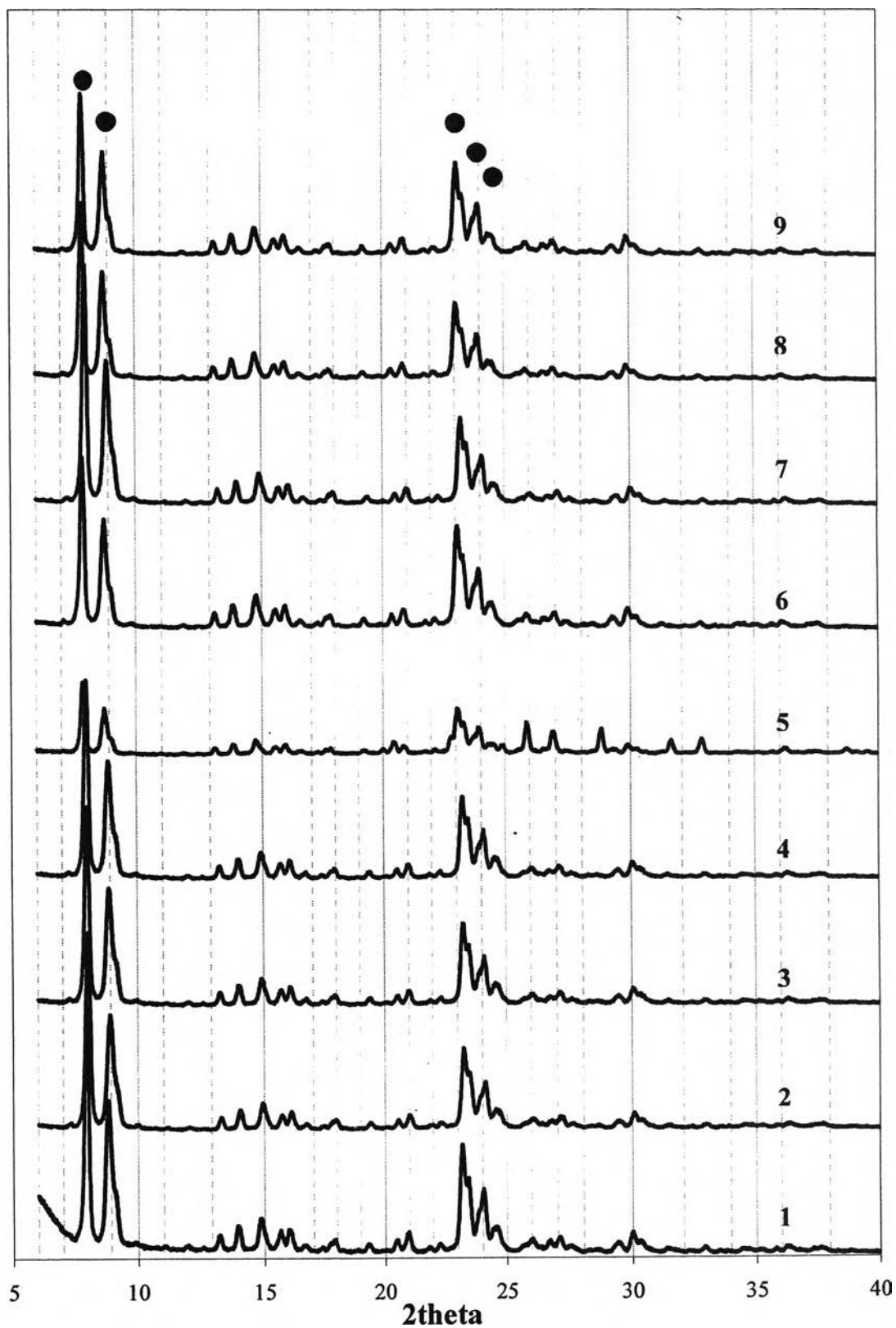
Figure 5.1 XRD patterns of TS-1 ratio60 (1), ratio40 (2), ratio32 (3), ratio22 (4) and the pretreatment with 5 M \text{HNO}_3 ratio60 (5), ratio40 (6), ratio32 (7), ratio22 (8) and the pretreatment with 3 M \text{HNO}_3 ratio40 (9).
