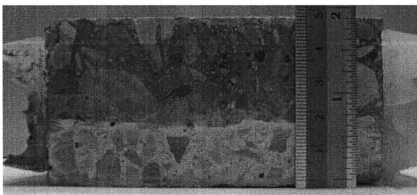
Figure B.6 Chloride penetration depth of specimen with replacement by 25% fly ash and w/b = 0.5 (case F2)
