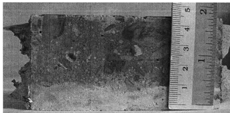
Figure A.6 Chloride penetration depth of specimen with replacement by 35% fly ash and w/b = 0.4 (case D7)
