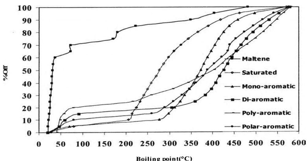
**Table G3** True boiling point curves of non-catalytic pyrolysis
