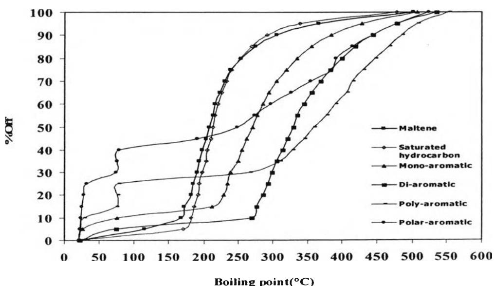
**Table G9** True boiling point curves of catalytic pyrolysis
