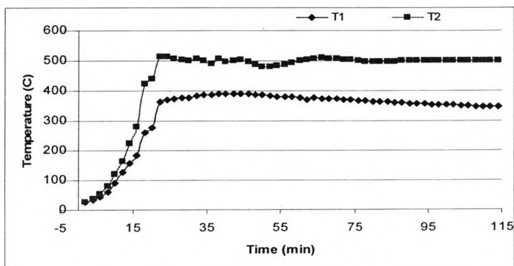
**Table A16** Operating temperatures, (0.50 wt % Pd/H-BETA , Ion-exchange):
