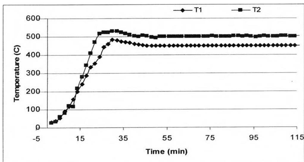
**Table A15** Operating temperatures, (0.25 wt % Pd/H-BETA , Ion-exchange):
