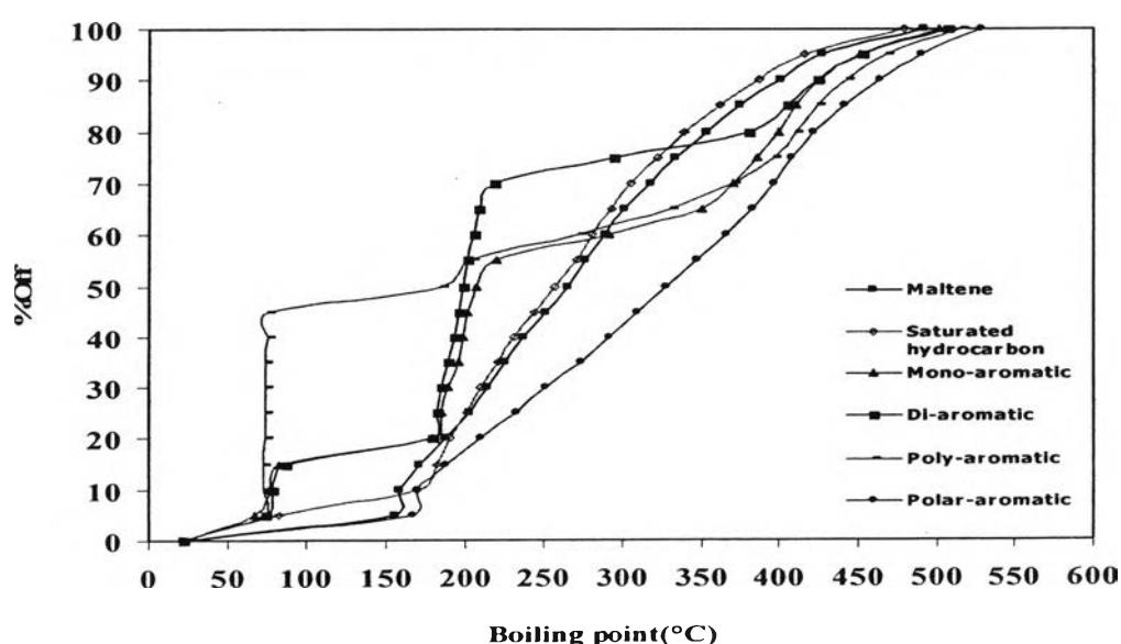
**Table G4** True boiling point curves of catalytic pyrolysis
