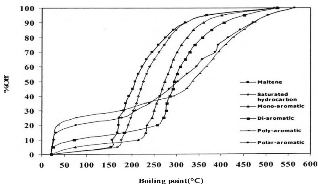
**Table G5** True boiling point curves of catalytic pyrolysis
