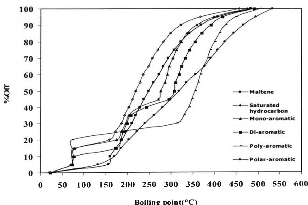
**Table G15** True boiling point curves of catalytic pyrolysis
