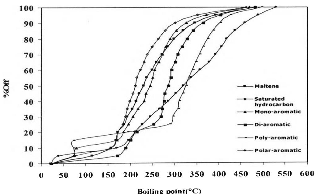
**Table G11** True boiling point curves of catalytic pyrolysis
