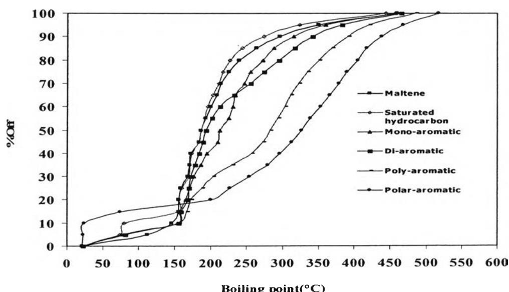
**Table G6** True boiling point curves of catalytic pyrolysis
