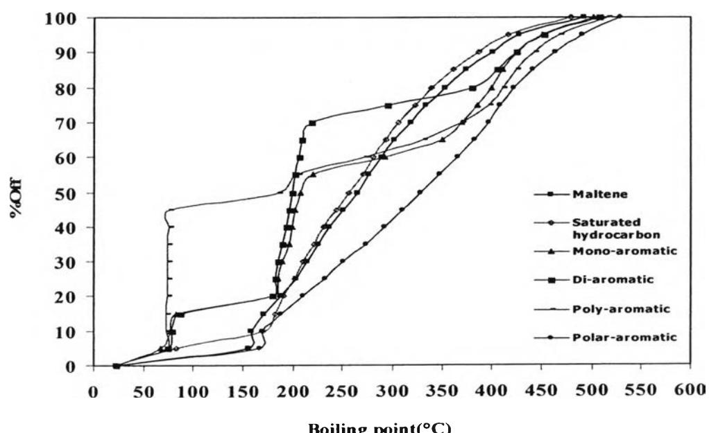
**Table G10** True boiling point curves of catalytic pyrolysis
