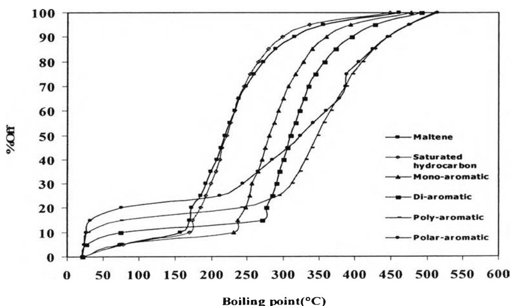
**Table G8** True boiling point curves of catalytic pyrolysis
