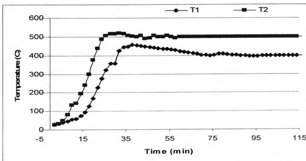
**Table A10** Operating temperatures, (0.25 wt % Pd/H-BETA, Cat temp 450°C):
