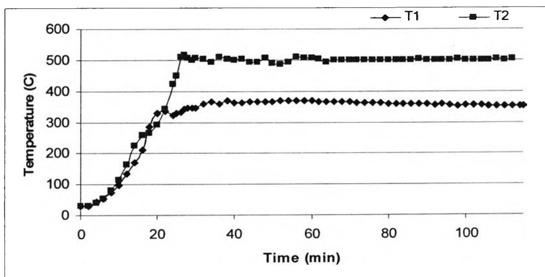
**Table A9** Operating temperatures, (0.25 wt % Pd/H-BETA, Cat temp 400°C) :
