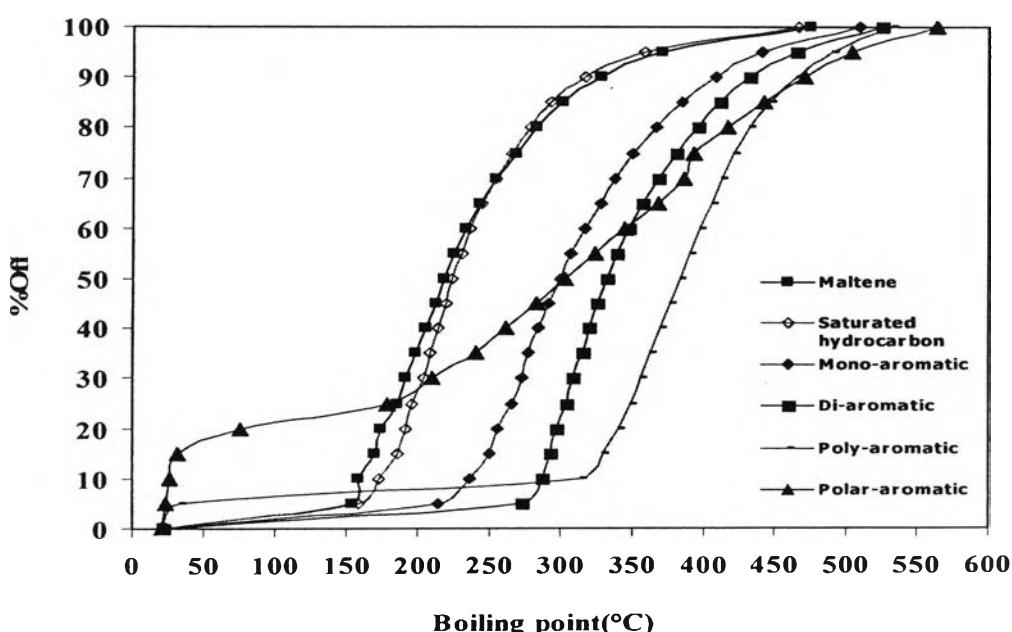
**Table G7** True boiling point curves of catalytic pyrolysis
