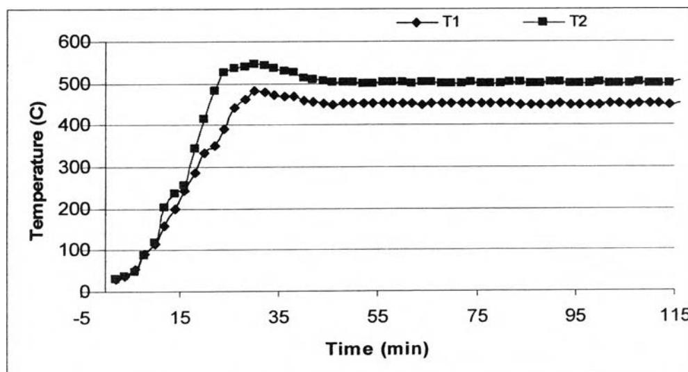
**Table A11** Operating temperatures, (0.25 wt % Pd/H-BETA, Cat temp 500°C):
