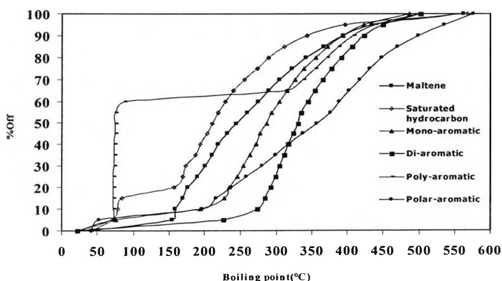
**Table G2** True boiling point curves of non-catalytic pyrolysis
