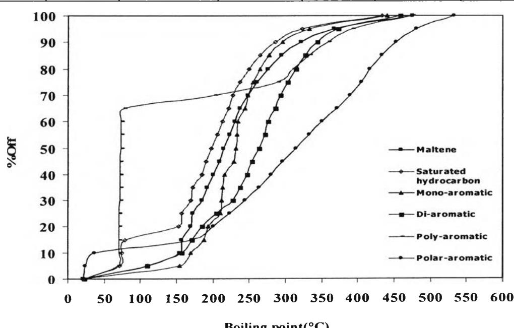
**Table G14** True boiling point curves of catalytic pyrolysis
