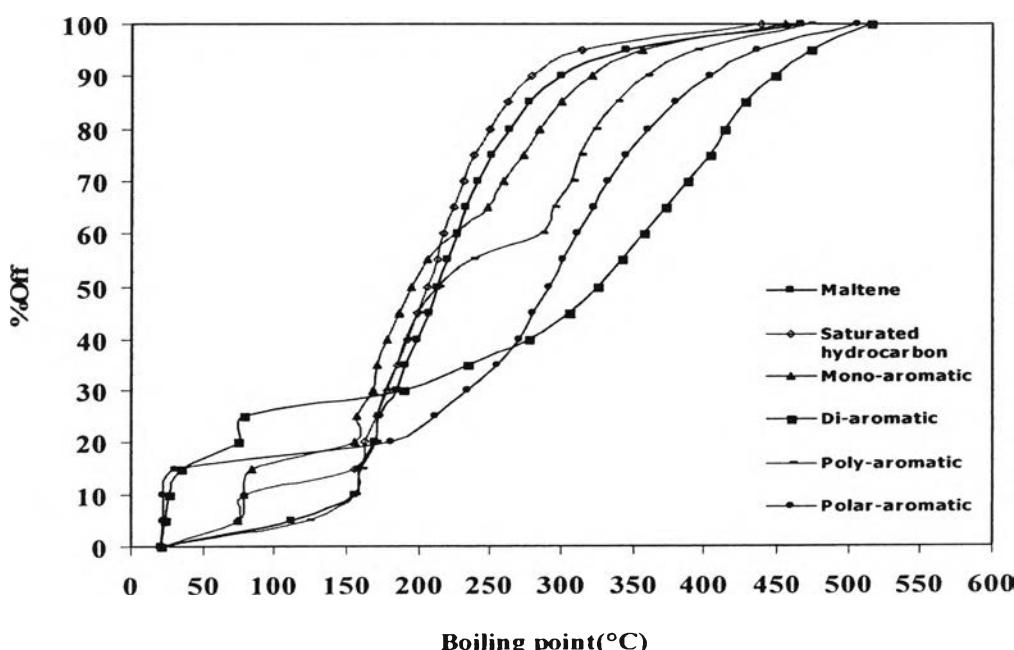
**Table G16** True boiling point curves of catalytic pyrolysis
