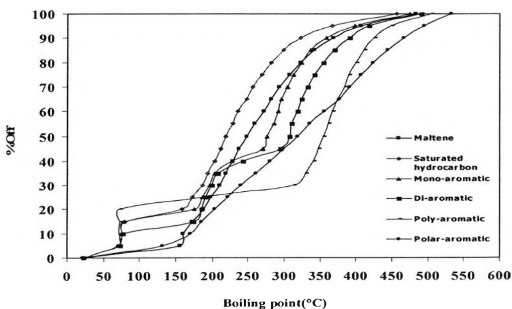
**Table G12** True boiling point curves of catalytic pyrolysis
