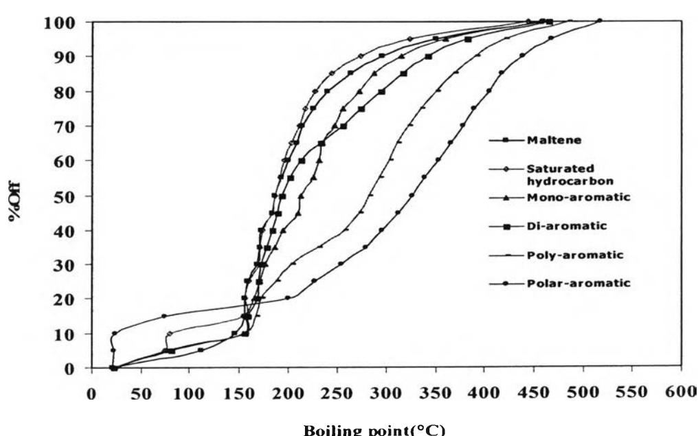
**Table G17** True boiling point curves of catalytic pyrolysis
