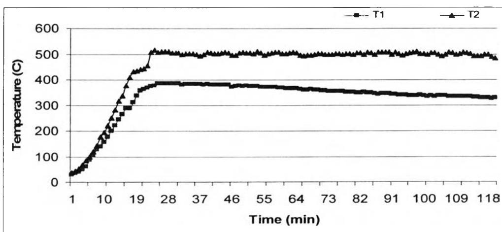
**Table A2** Operating temperatures, non catalytic pyrolysis (Catalytic temp. 350°C):
