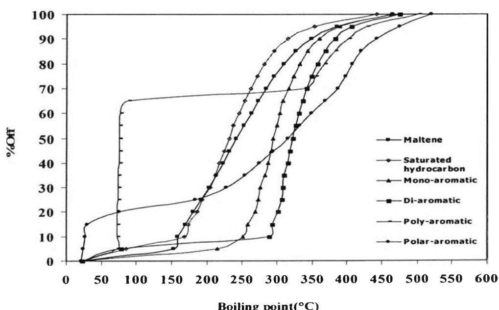
**Table G13** True boiling point curves of catalytic pyrolysis
