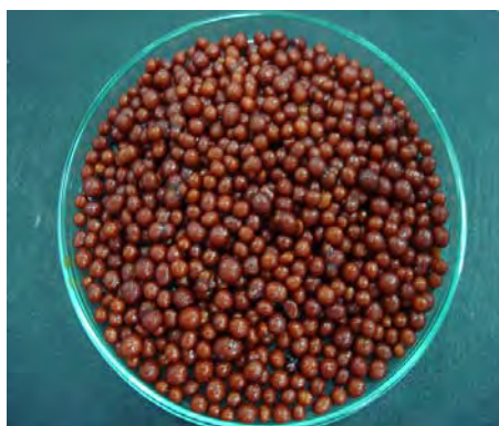
Figure 4.8 Urea fertilizers encapsulated with pre-cured oil.
