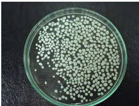
Figure 4.2 Uncoated urea fertilizers in DI water at 1 minute.
