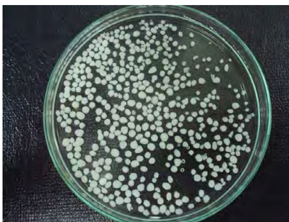
Figure 4.3 Uncoated urea fertilizers in DI water at 2 minutes.
