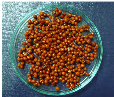
Figure 4.7 Urea fertilizers encapsulated with drying oil by pan coater.
