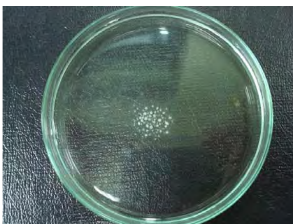
Figure 4.4 Uncoated urea fertilizers in DI water at 3 minutes.
