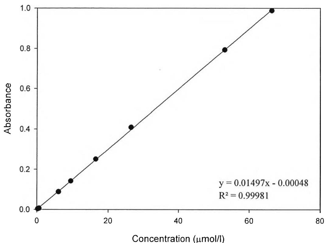
**Figure D2** Calibration curve of SDBS solution.
