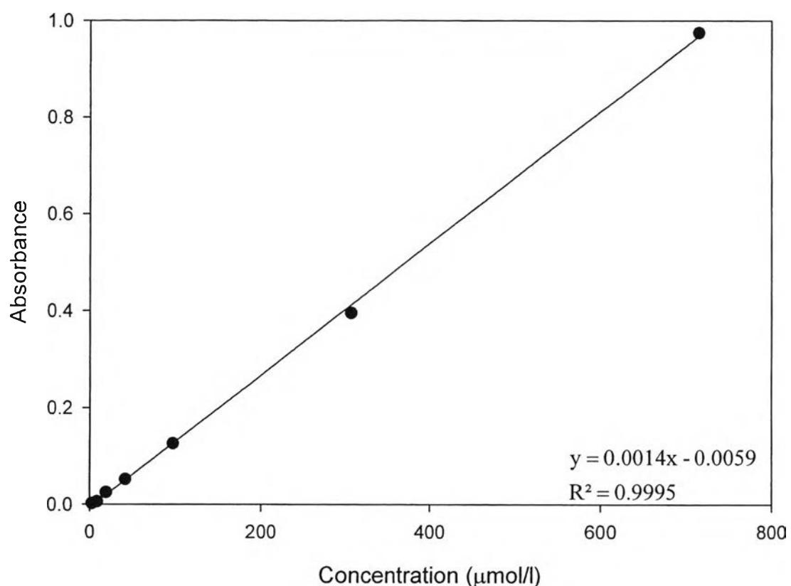
**Figure D3** Calibration curve of OP(EO)<sub>10</sub> solution.
