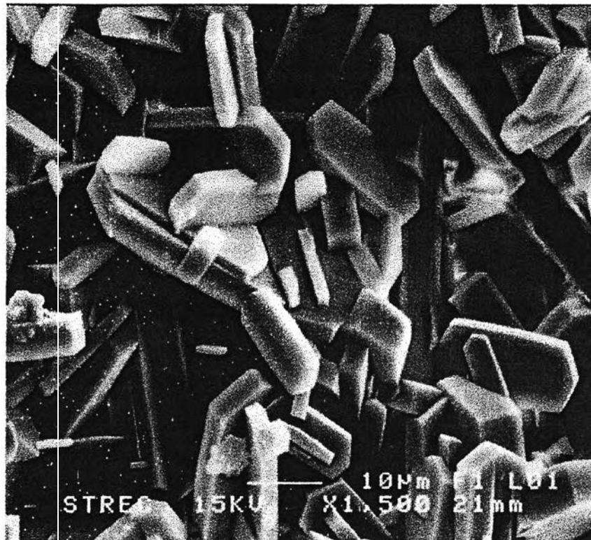
Figure 4.9 SEM image of silicalite membrane on borosilicate disc support.
