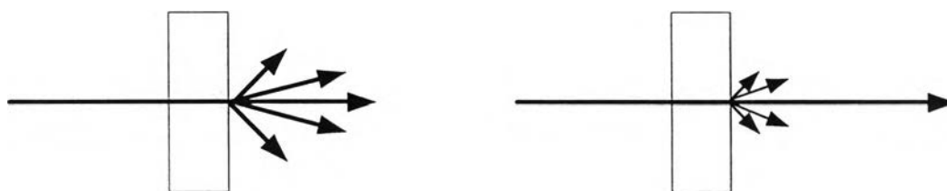
Figure 3.1 The light transmission of (a) large-grained PCA (translucent) with high diffuse transmission and a low in-line transmission and (b) fine-grained PCA (transparent) with a low diffuse transmission and a high in-line transmission.
