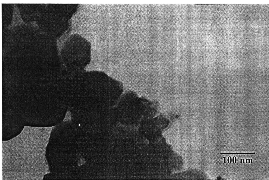
Figure 5.20(b) TEM photograph of the product at Zn/Al=1.00 synthesized in toluene after calcination at 1100°C.
