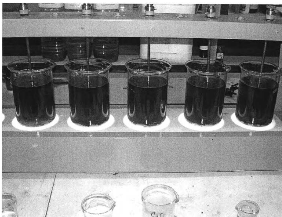
Figure B.9 Jar test experiment.
