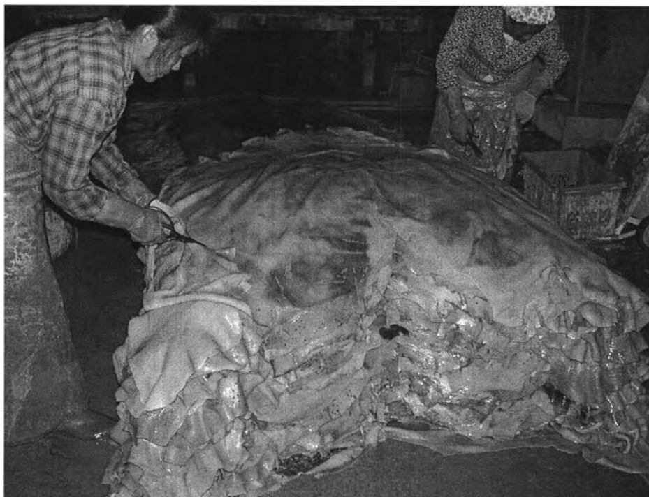
Figure B.3 Trimming and decorating before Chrome tanning.
