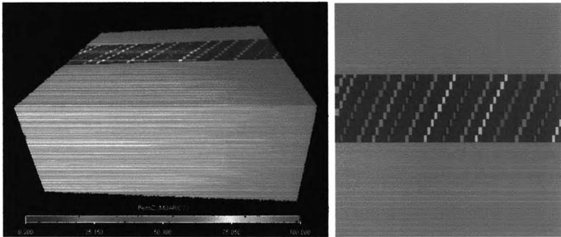
Figure 3.2: 3-D illustration and top view of reservoir model showing the heterogeneity of permeability.
