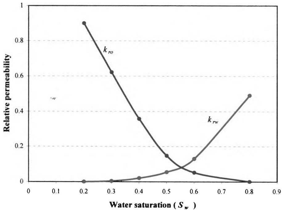
Figure 3.5: Relative permeability respect to water saturation.
