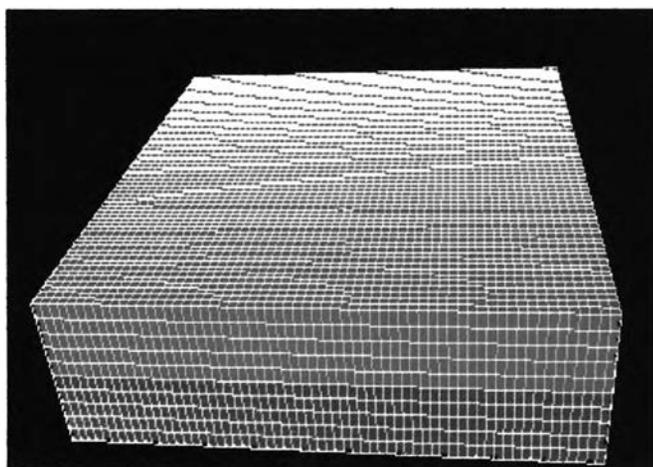
Figure 3.1: Reservoir grid cell model.
