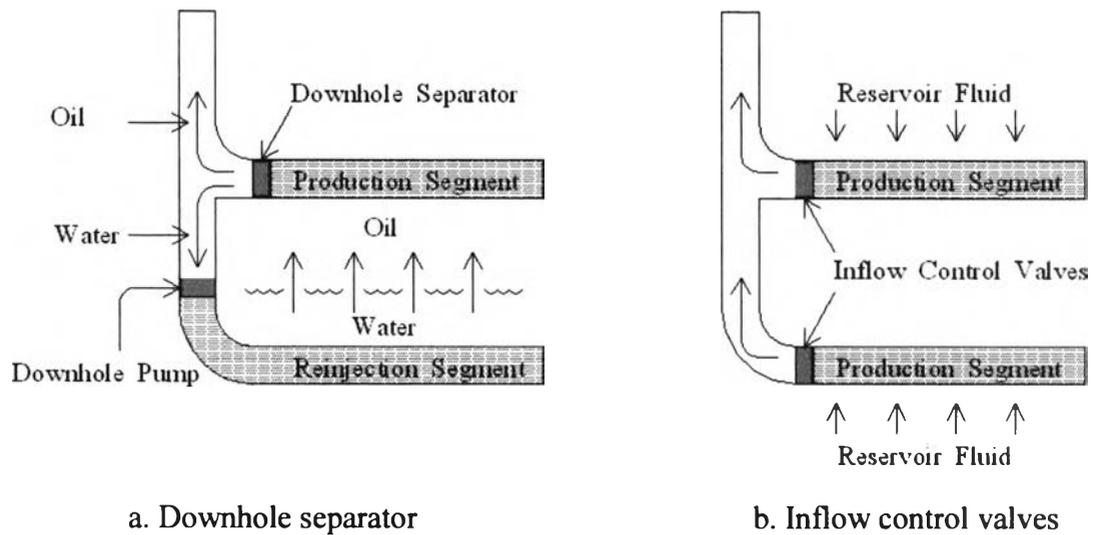
Figure 3.10: Schematic diagrams of multi-segment option.
