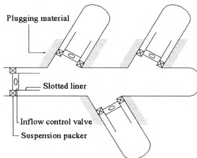
Figure 3.9: Intelligent completion system.
