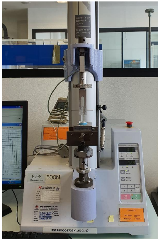
Figure 13 Specimen placed in the testing machine for the tensile bond strength test.
