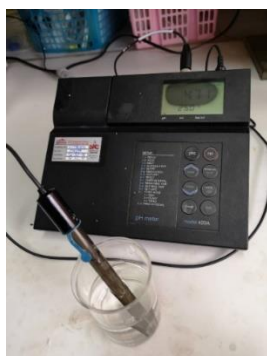
Figure 25 pH adjustment of the solution using pH meter (Orion 420A)
