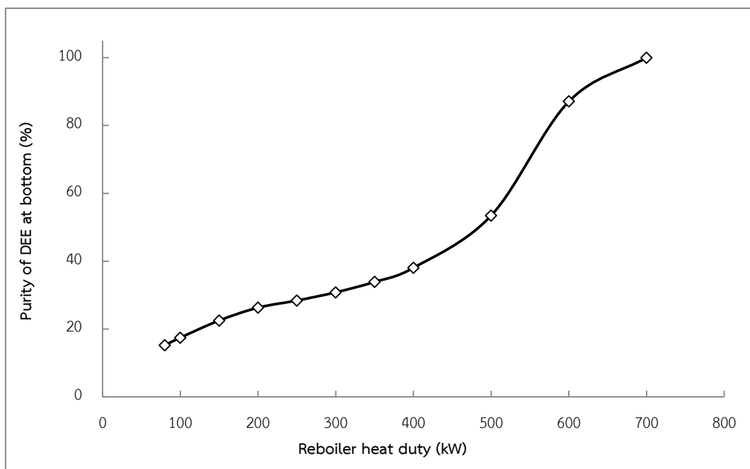
Figure 23 Simulation results of the effect of reboiler heat duty on purity of DEE
