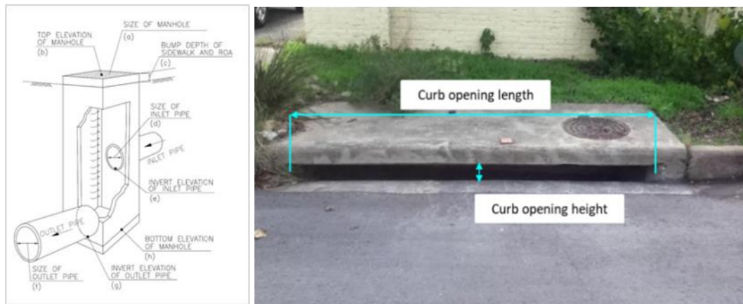
Figure 4-7: Manhole components and detail of Curb Opening Inlet at Grade of the manhole
