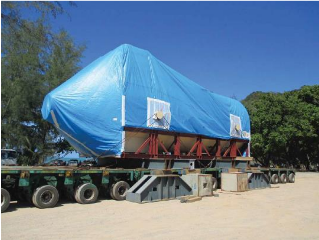
Figure 12 Generator transportation (Project D monthly reports)
