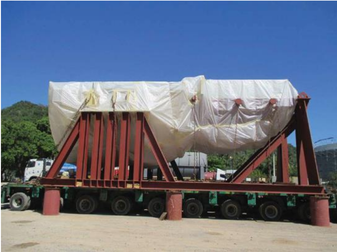
Figure 14 Steam turbine's lower casing transportation (Project D monthly reports)
