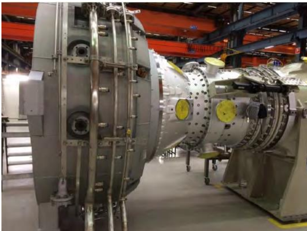
Figure 11 Gas turbine fabrication in manufacturer workshop (Project C monthly reports)
