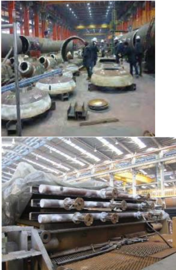
Figure 13 HRSGs fabrication in manufacturer workshop (Project C monthly reports)
