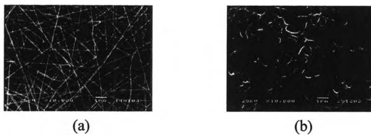
Figure 1. The scanning electron micrographs of electrospun fibers of PA-6 in a single solvent: a) 85 wt.% formic acid; and b) m -cresol (10,000x).
