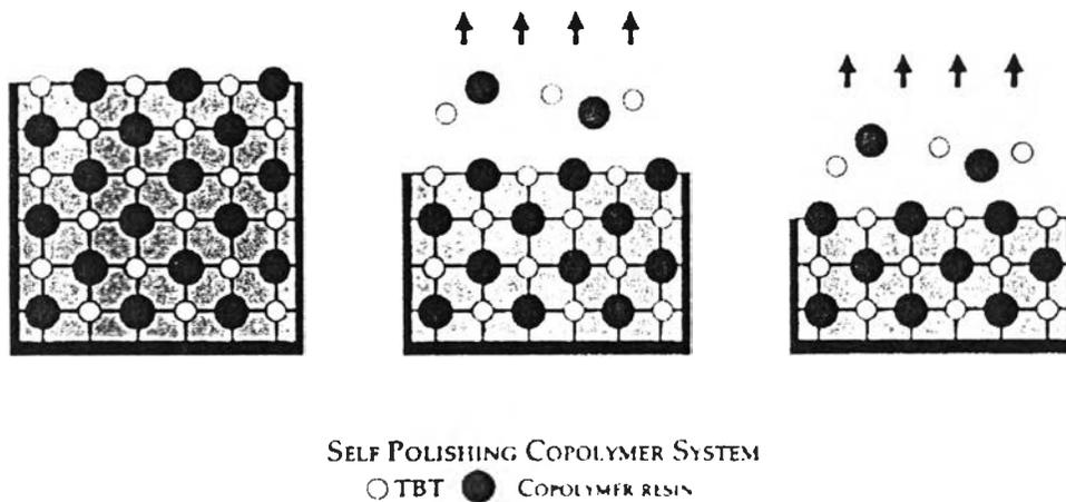
At the point surface sea water hydrolyses the TBT copolymer bond and the TBT biocide and copolymer resin is slowly released at a controlled rate. A uniform anti-fouling performance is achieved throughout the life of the paint.
