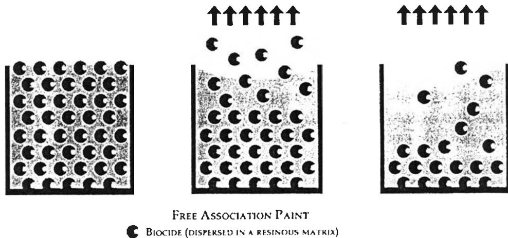
The biocide leaches freshly from the resinous matrix. The initial release is rapid and uncontrolled. Subsequent release declines steadily from the matrix such that the anti-fouling performance of the paint diminishes with time.
