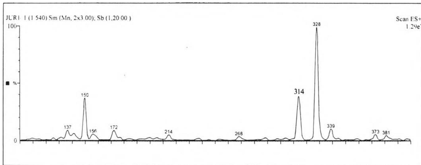
**Figure 22** Mass spectrum of 1,2-dehydronorreticuline (LC-MS, APCI)
