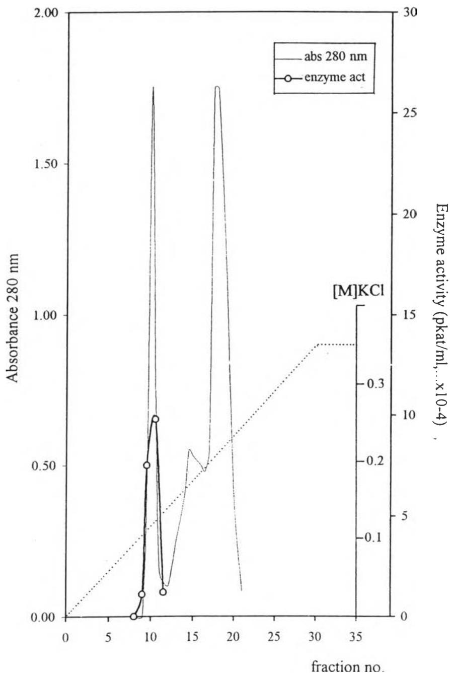
**Figure 27** The first MonoQ HR 5/5 anion exchange chromatography of the enzyme from DEAE-Sephacel column
