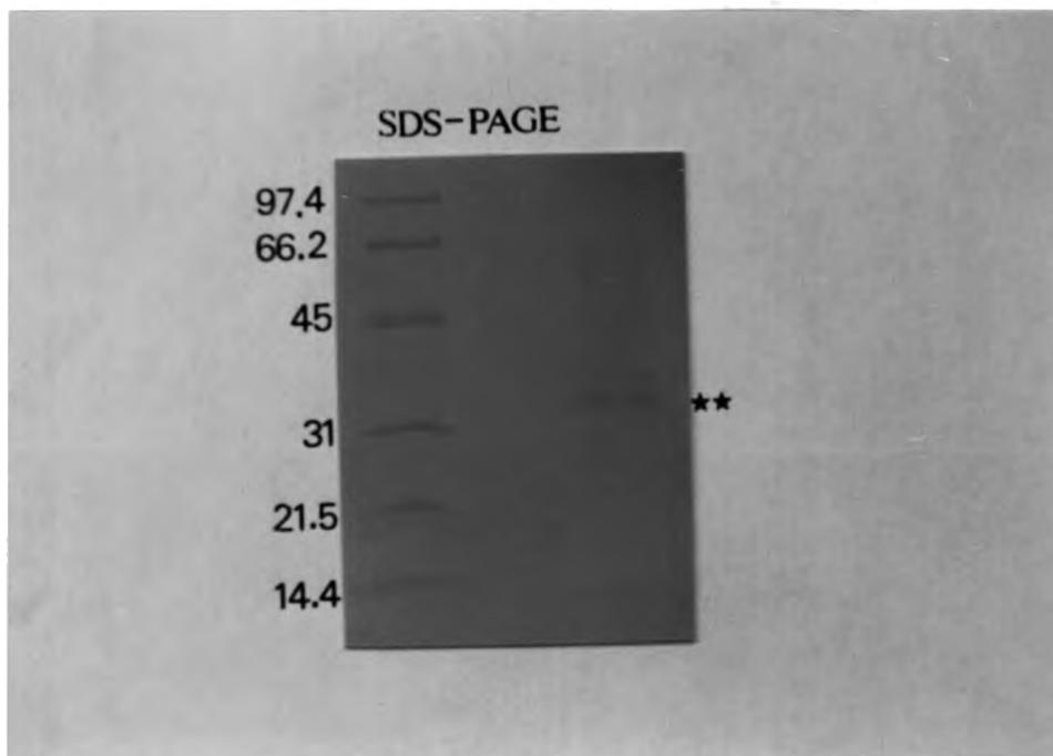
**Figure 33** SDS-PAGE of purified enzyme (Coomassie blue staining)
