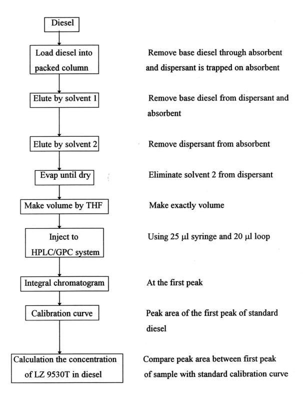
Scheme 3.2 The overall process to determine the concentration of LZ 9530T as dispersant additive in diesel
