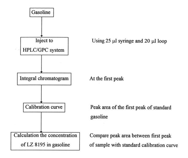
Scheme 3.1 The overall process to determine the concentration of LZ 8195 as dispersant additive in gasoline
