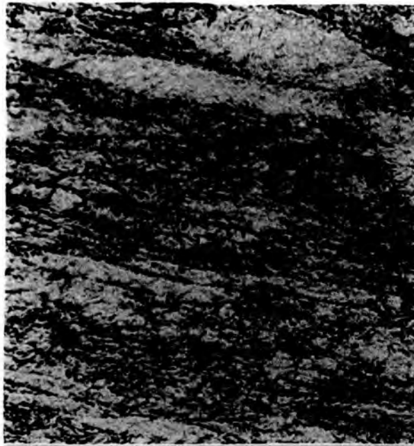
(e) Rolled 70% in nonrecrystallization region (200x)
