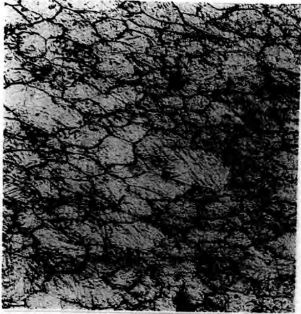
(a) Rolled 30% in nonrecrystallization region (100x)
