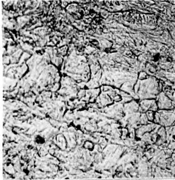
(e) Rolled 70% in nonrecrystallization region (500x)
