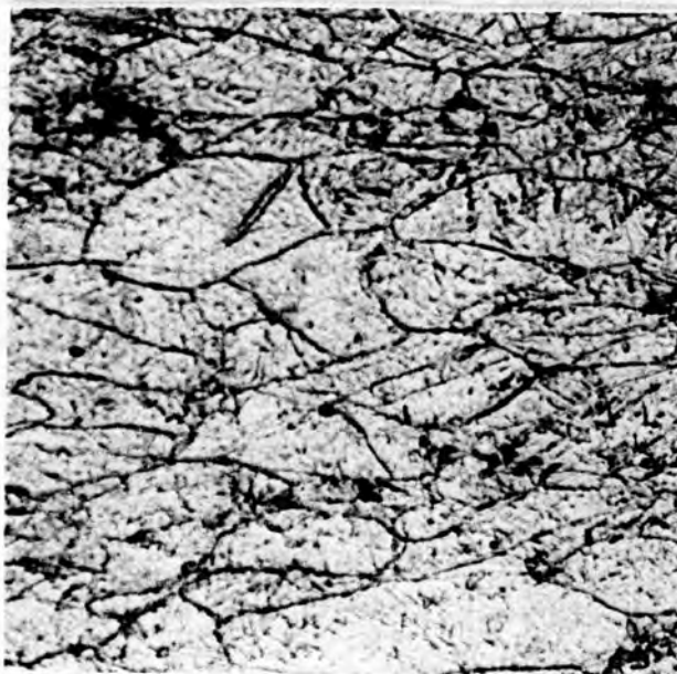
(b) Rolled 40% in nonrecrystallization region (200x)
