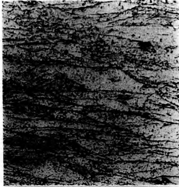
(e) Rolled 70% in nonrecrystallization region (200x)
