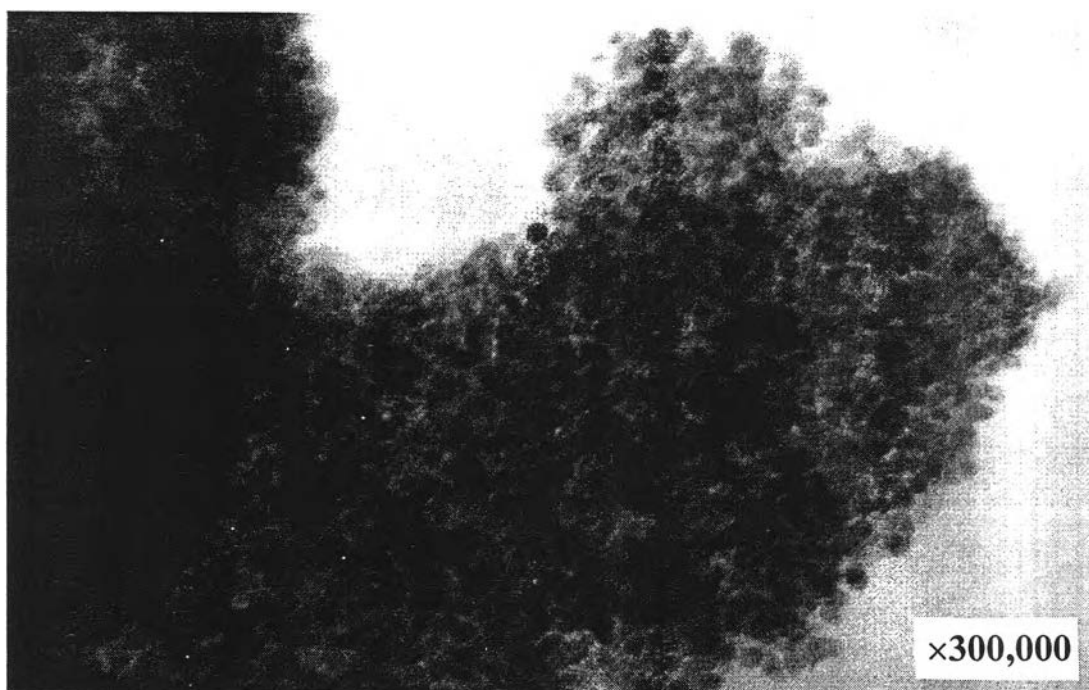
Figure 5.12(e) TEM photograph of silica modified titanium (IV) oxide with Si/Ti = 0.5 synthesized by 2-propanol.
