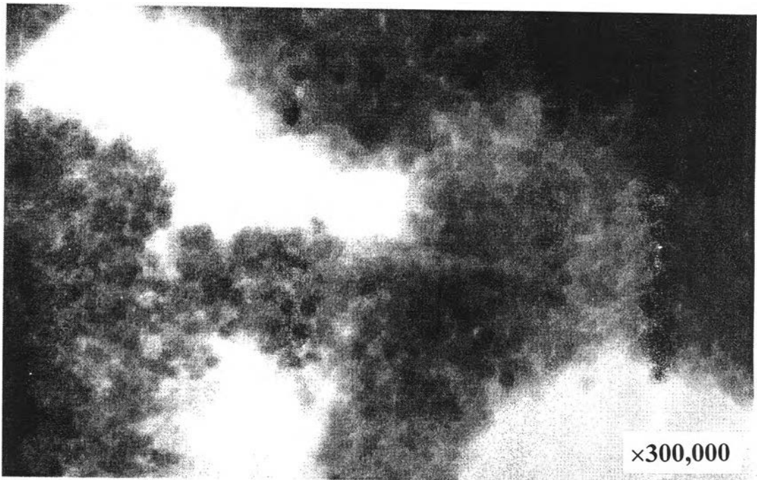
Figure 5.8(e) TEM photograph of silica modified titanium (IV) oxide with Si/Ti = 0.5 synthesized by 1,4 butanediol.
