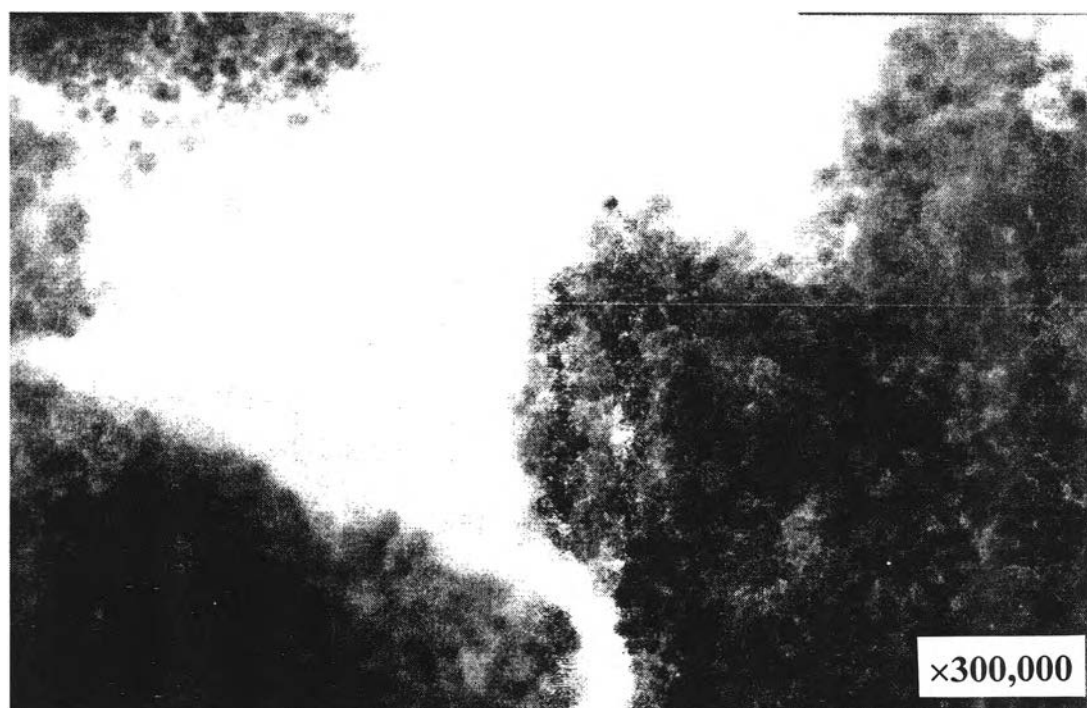
Figure 5.8(d) TEM photograph of silica modified titanium (IV) oxide with Si/Ti = 0.3 synthesized by 1,4 butanediol.
