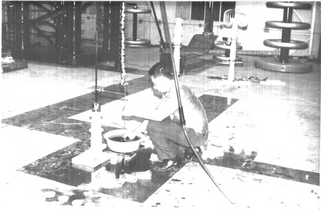
12. Dielectric Strength-break down test.
