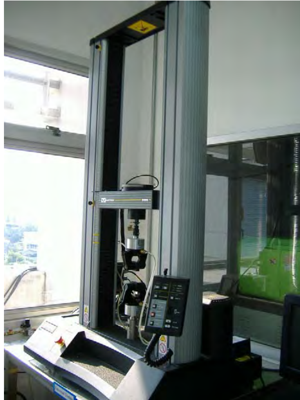
Figure 4.9 Universal Testing Machine equipment
