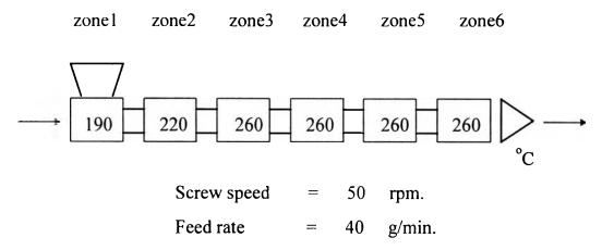
The extrudate was cooled in the water (~25  $^{\circ}$ C) and cut into pellets form by a Planetrol 07502 pelletizer.
