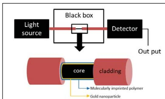
Figure 15 SPR spectrometer configuration
