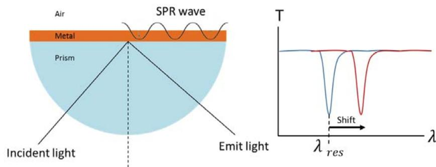
**Figure 3** Kretschmann's configuration of SPR spectroscopy
