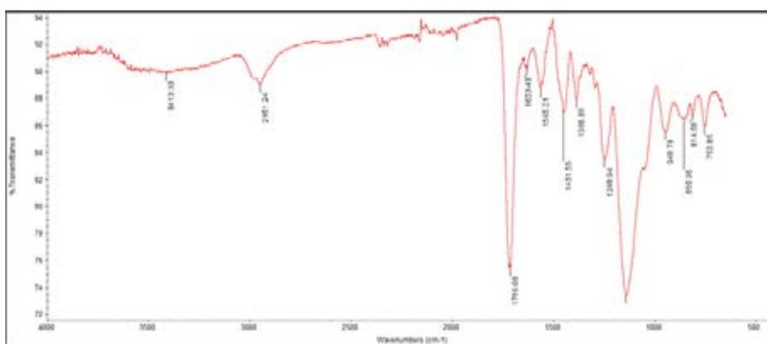
Figure 32 IR spectrum of MIP synthesized via thermal polymerization method
