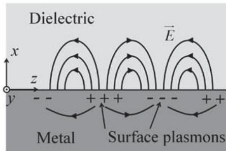
**Figure 1** Surface plasmon propagation along the interface between electric and dielectric surface [9]
