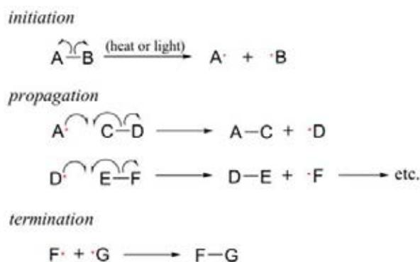
Figure 6 Three steps of polymerization [15]
