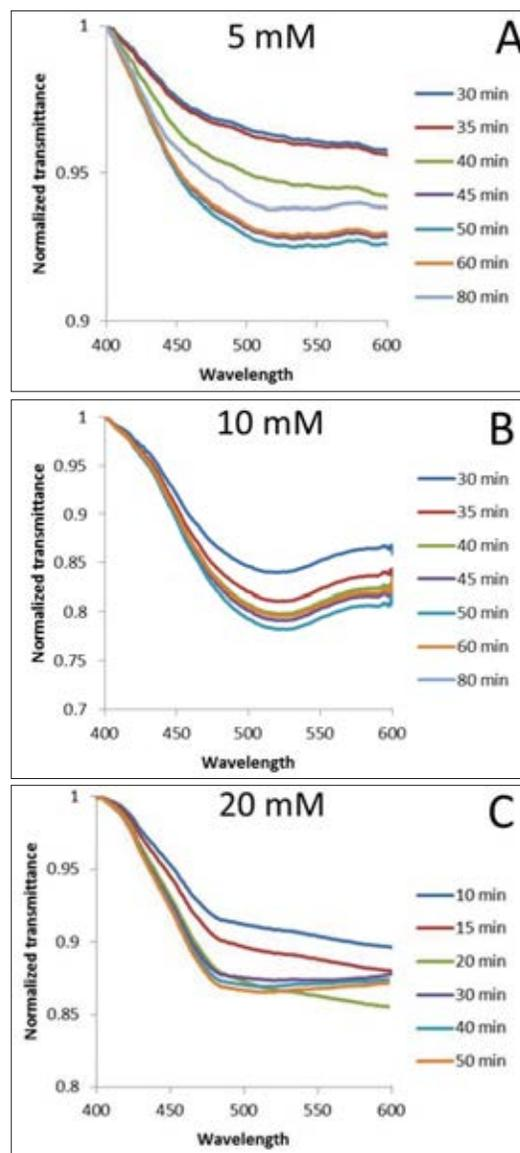
**Figure 16** The SPR signals obtained from optical fibers deposited with gold nanoparticles at various concentrations of gold chloride at various immersion times (A) 5 mM of at 30-80 min (B) 10 mM at 30-80 min and (C) 20 mM at 10-50 min.
