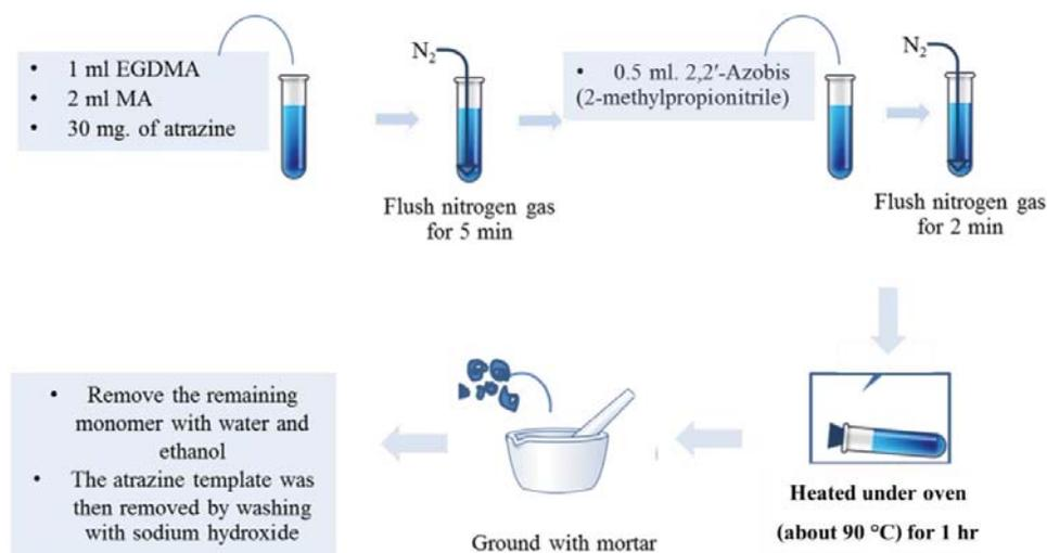
**Figure 11** Synthesis of molecularly imprinted polymer via thermal polymerization method
