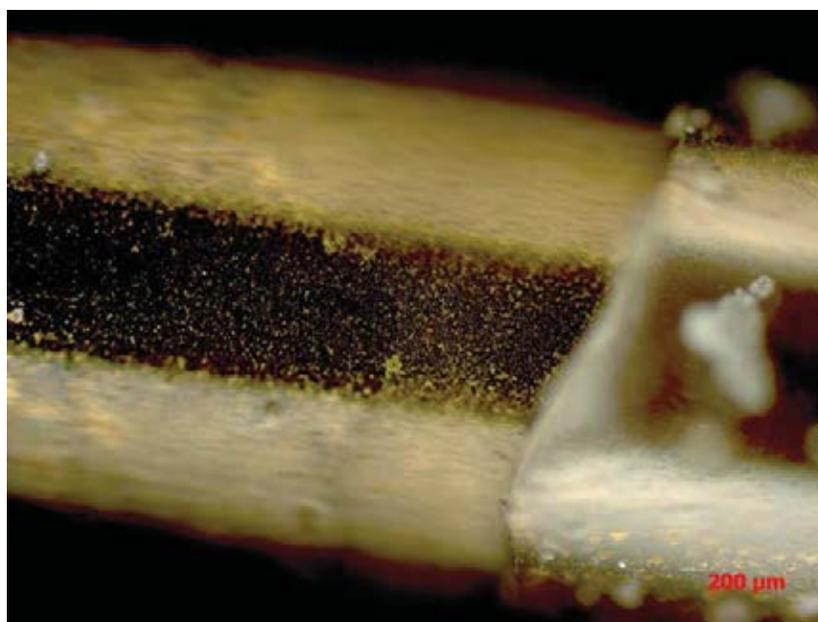
Figure 30 The image of SPR probe assembly 10 mM with gold nanoparticle for 60 min
