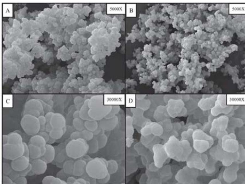
**Figure 20** SEM images of MIP (A and C) and NIP (B and D) synthesis via atom transfer radical polymerization technique using 2-bromopropionate as initiator
