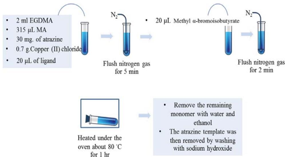
**Figure 13** Synthesis of molecularly imprinted polymer via ATRP method
