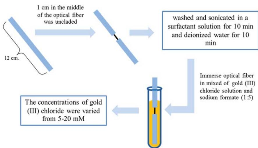
**Figure 10** The process of self-assembly of gold nanoparticle on the surface of the optical fiber
