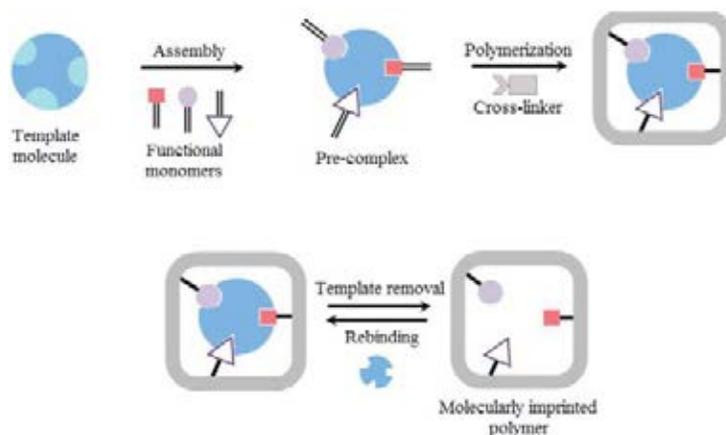
**Figure 5** The principle steps of molecular imprinting polymer polymerization [14]
