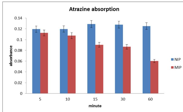
**Figure 21** Amounts of atrazine standard in the solution after treated with MIP and NIP (via ATRP method) at various time, using 0.1 g of polymer and 30 ppm as initial concentration of atrazine
