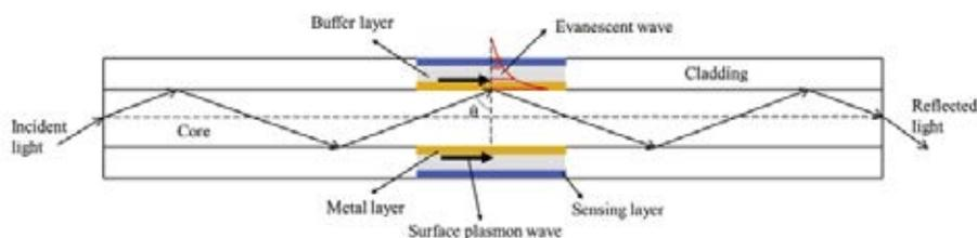
**Figure 4** Optical fiber SPR spectroscopy [12]
