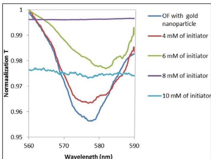
Figure 25 The SPR signal of the SPR probe using various concentration of initiator
