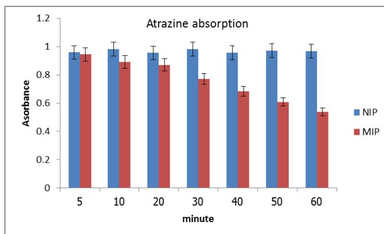
**Figure 19** Amounts of atrazine standard in the solution after treated with MIP and NIP (via thermal polymerization method) at various time, using 0.1 g of polymer and 30 ppm as initial concentration of atrazine
