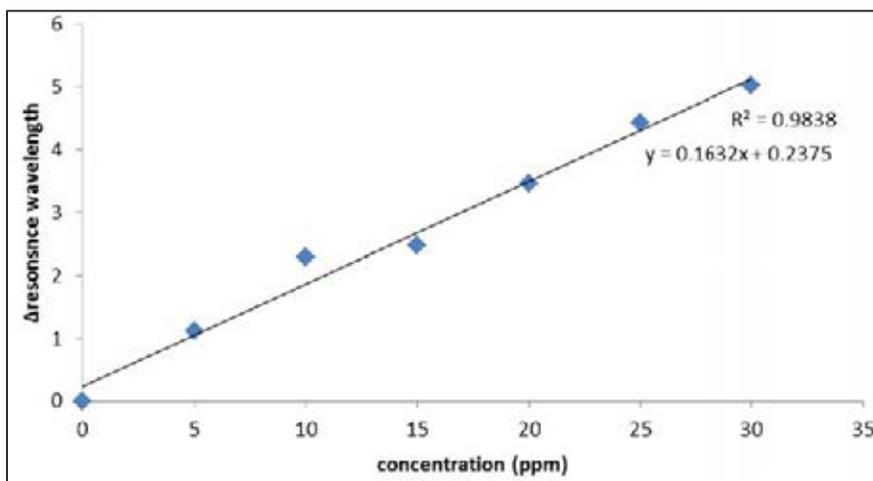
**Figure 28** Calibration curve of atrazine obtained from SPR probe modified with MIP via ATRP method
