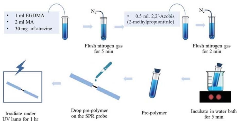
**Figure 12** Assembly of MIP on the optical fiber using thermal/UV-polymerization
