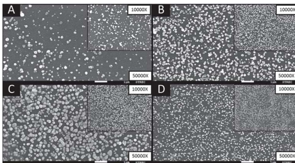
**Figure 17** SEM images of the optical fiber surfaces using gold chloride concentration of 10 mM at different immersion time; (A) 35 min, (B) 50 min (C) 60 min and (D) 80 min
