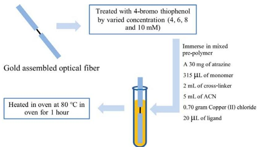
Figure 14 Assembly of MIP on the SPR probe using modified ATRP method
