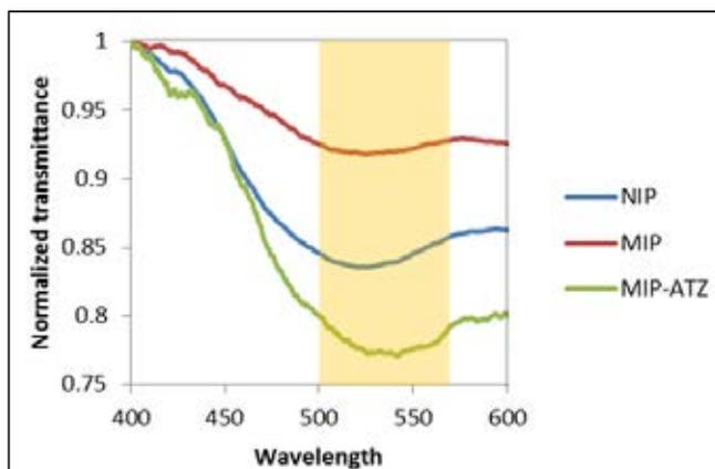
**Figure 24** Optical fiber SPR with MIP for sensing of atrazine (10 min soaking time, 5 mL of 30 ppm atrazine standard)
