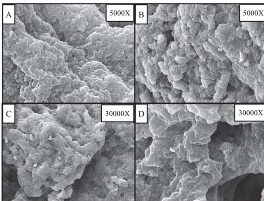
**Figure 23** SEM images of MIP (A and C) and NIP (B and D) synthesis via atom transfer racial polymerization technique using 4-bromo thiophenol as initiator
