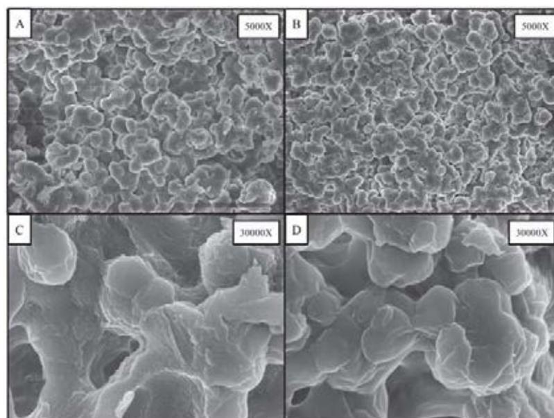
**Figure 18** SEM images of MIP (A and C) and NIP (B and D) synthesis via thermal polymerization technique
