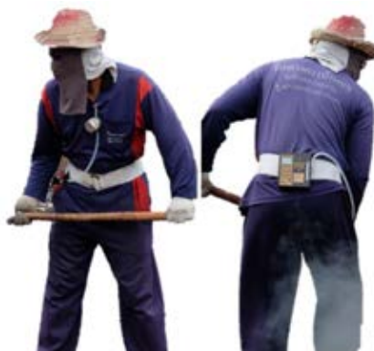
Figure 3.4 Installation of the personal air sampler equipment at worker's breathing zone
