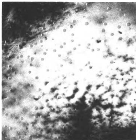
Figure 46 The picture should immiscible oil drop in the film of mouth refreshing film formula using HPMC polymer.
