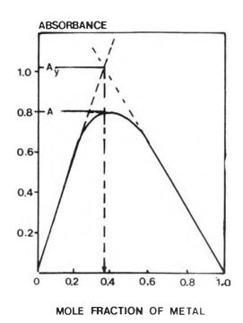
Fig B.1 Plot of Job's method for the 1:2 complex  $ML_2$
