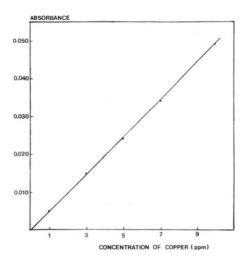
Fig E.1 Plot of Calibration on Cu-Salen complex at 562 nm, pH 4.5.
