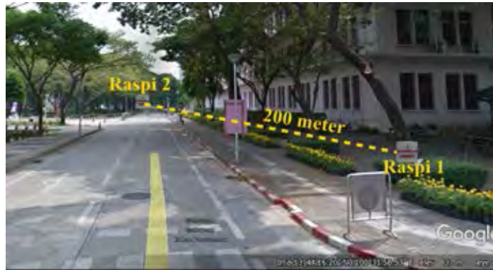
Figure 5.3: 200-metre wireless network reachability testing.
