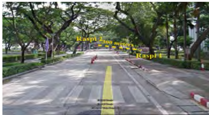
Figure 5.4: 300-metre wireless network reachability testing.
