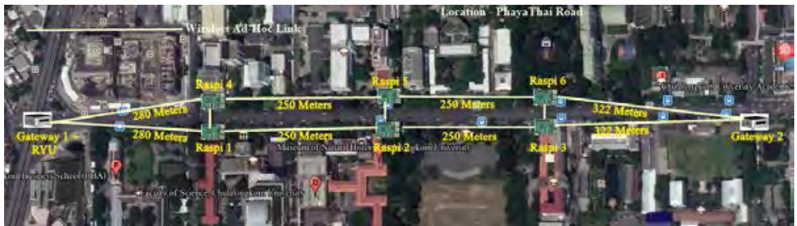
Figure 6.1: Topology of real outdoor SDWMN testbed on Phaya Thai road for road traffic monitoring network.
