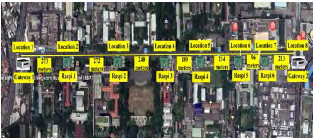
Figure 3.1: Typical installation scenario of outdoor SDWMN to monitor road network traffic (e.g. on Phaya Thai road, Bangkok).
