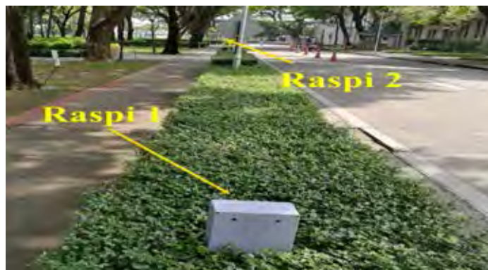
Figure 5.2: 100-metre wireless network reachability testing.
