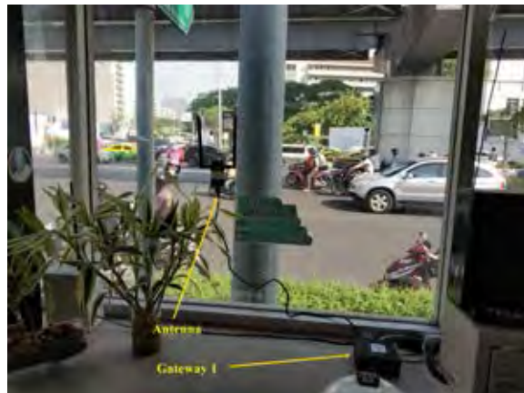
Figure 6.6: Traffic police box near Sam Yan MRT station on Rama 4 road where Gateway 1 is installed.
