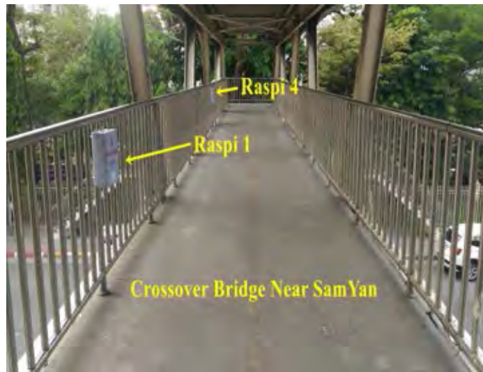
Figure 6.5: Position of wireless mesh node over crossover bridge on Phaya Thai Road.
