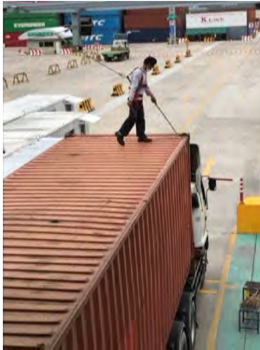
Figure 8 Haulage company's operator inspect roof of container with safety device at his back (TPAS's container round use system project, 2019)
