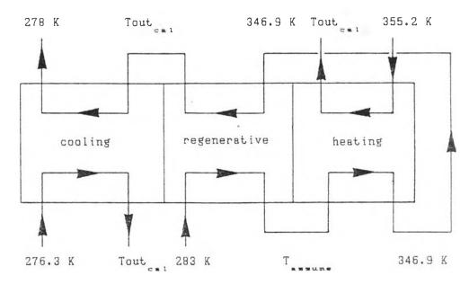
The computer code can be used to calculate the number of therm plates of the heating section and the regenerative section by
