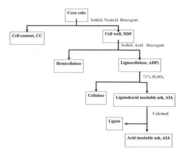
Figure A1 Schematic of detergent analysis procedure flow diagram.
