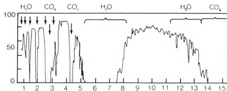
Fig. 1 Transmission versus wavelength for 1 mile of air. Water and carbon dioxide absorption bands are indicated.
