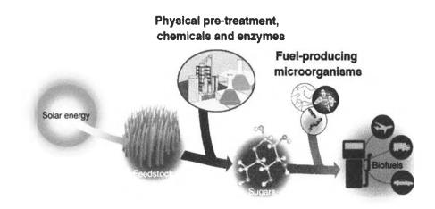
Figure 1.1 Biofuels production from lignocellulosic biomass (Cascone, 2008).
