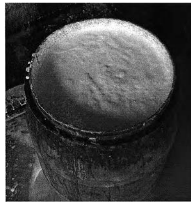
Figure 3.1. The fresh field latex contained in plastic container was preserved with ammonium hydroxide as a preservative.
