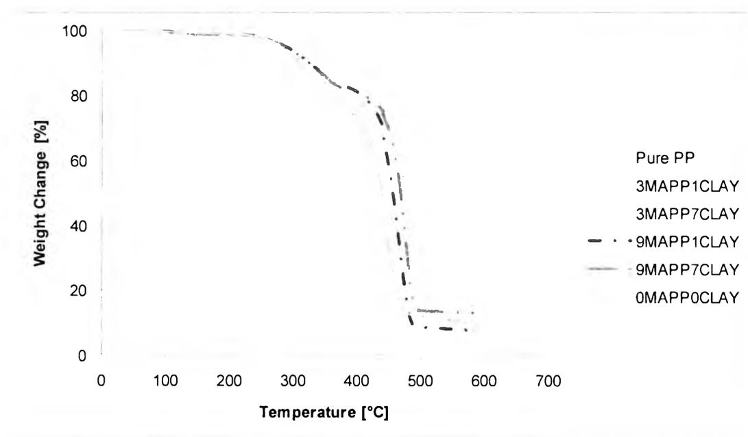
**Figure 4.8** Effect of nanoclay and MAPP content on thermal stability of nanoclay incorporated wood plastic composites.
