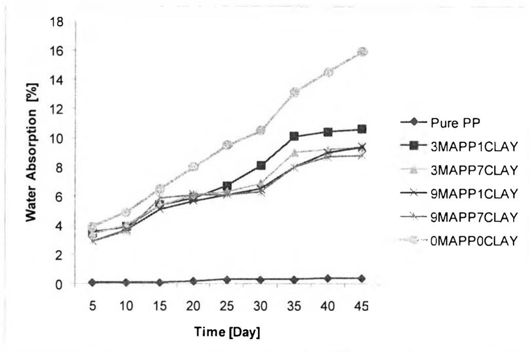
**Figure 4.10** Effect of nanoclay and MAPP content on water uptakes of nanoclay incorporated wood plastic composites.
