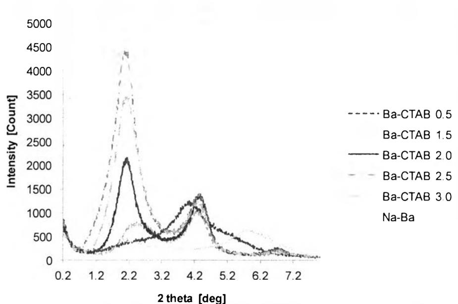
**Figure 4.1** XRD patterns of modified bentonite nanoclay at different CTAB levels and untreated bentonite.
