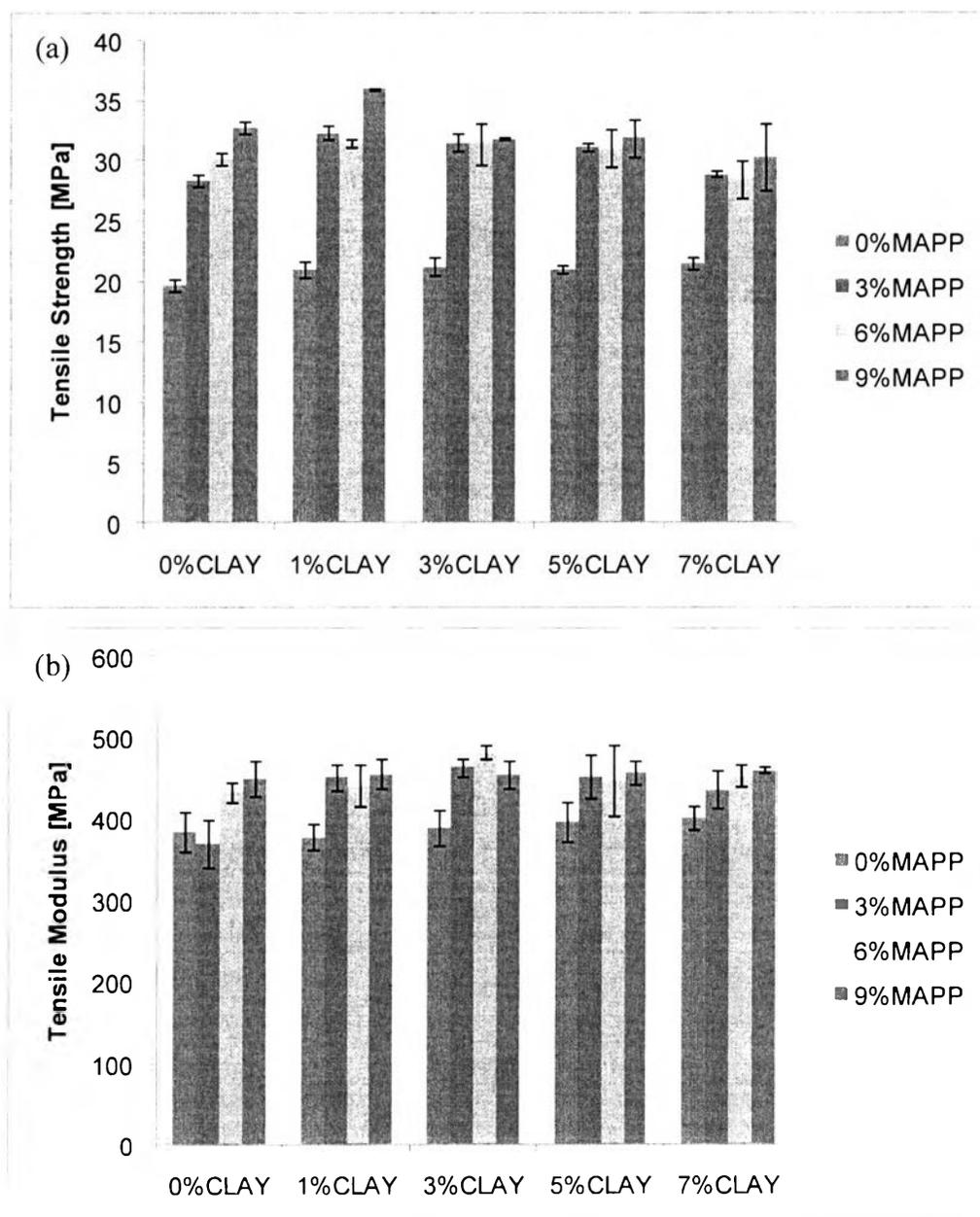
**Figure 4.2** Tensile strength (a) and tensile modulus (b) of WPC at nanoclay content of 0%, 1%, 3%, 5% and 7% w/w at different MAPP levels.
