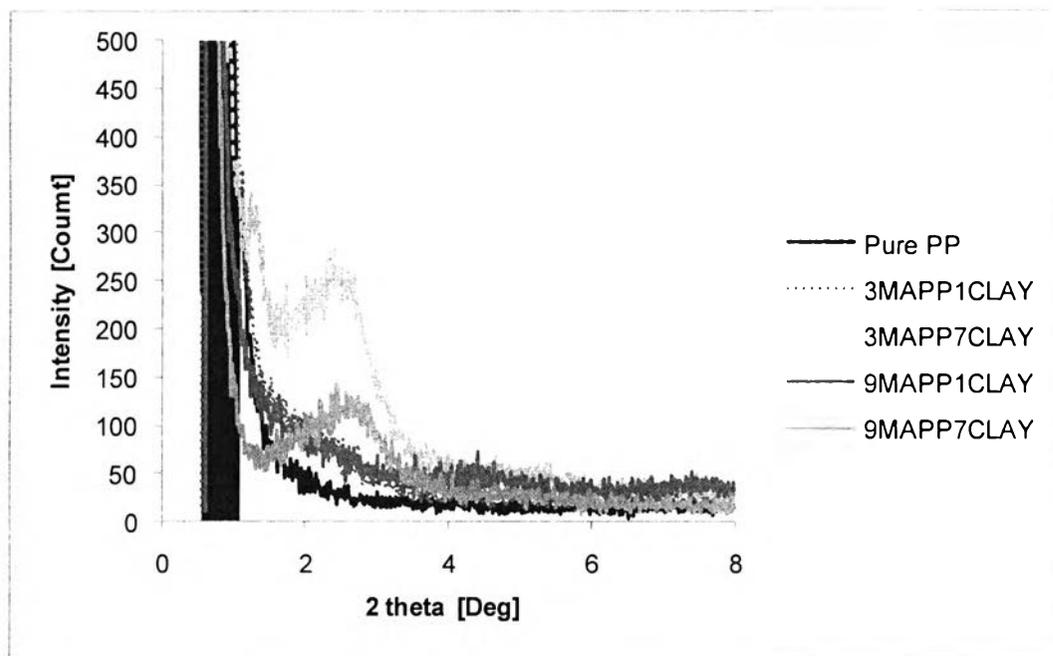
**Figure 4.9** XRD patterns of WPC at different CTAB levels and Nanoclay content.
