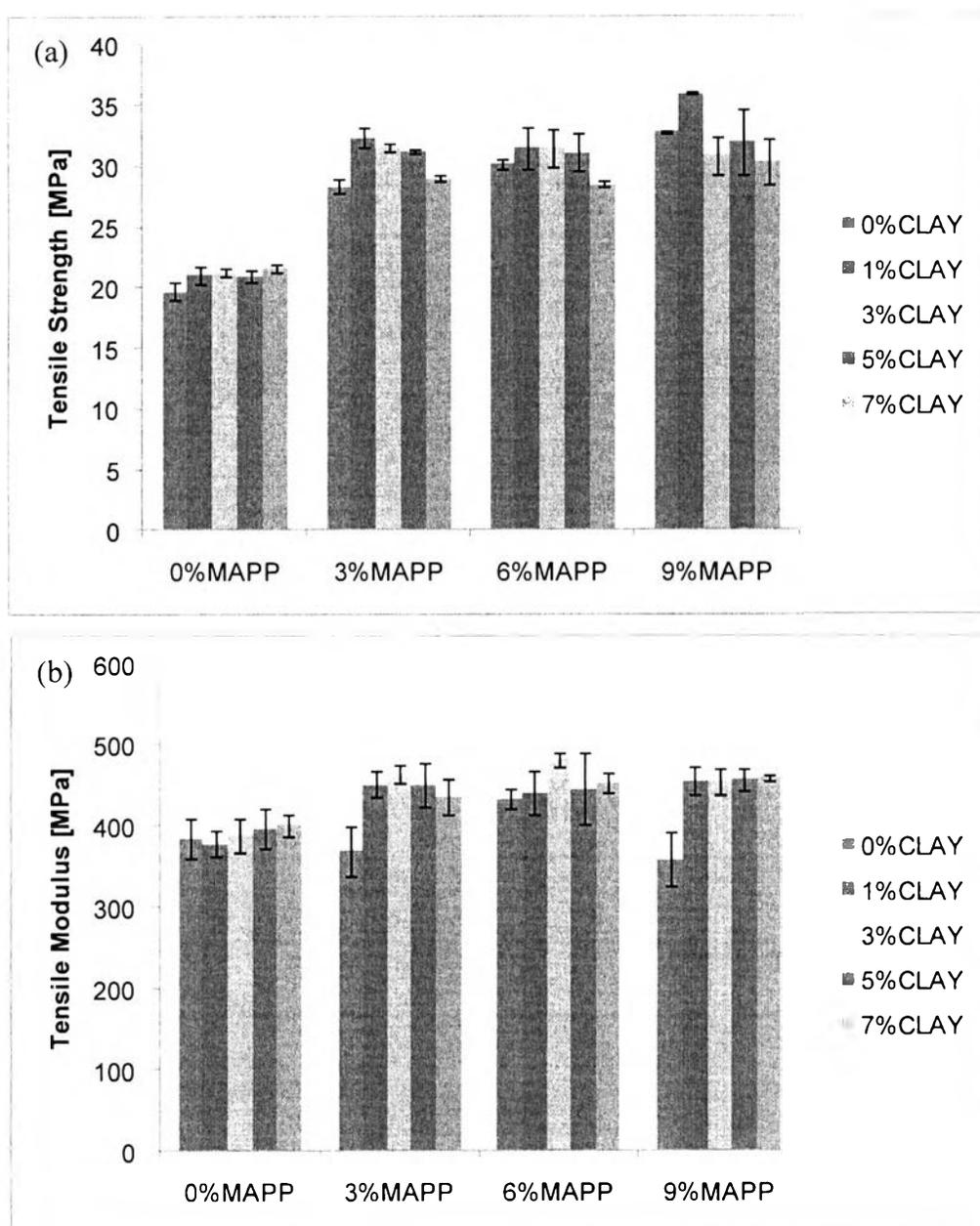
**Figure 4.5** Tensile strength (a) and tensile modulus (b) of WPC at MAPP content of 0%, 3%, 6% and 9% at different nanoclay levels.
