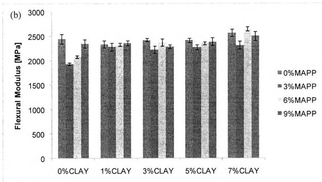
**Figure 4.3** Flexural strength (a) and flexural modulus (b) of WPC at nanoclay content of 0%, 1%, 3%, 5% and 7% w/w at different MAPP levels.
