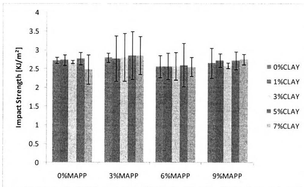
**Figure 4.7** Impact strength of WPC at MAPP content of 0%, 3%, 6% and 9% w/w at different nanoclay levels.
