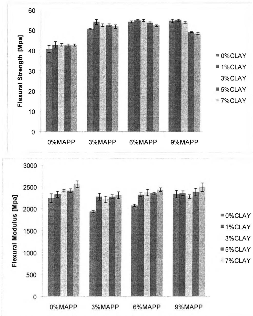
**Figure 4.6** Flexural strength (a) and flexural modulus (b) of WPC at MAPP content of 0%, 3%, 6% and 9% at different nanoclay levels.
