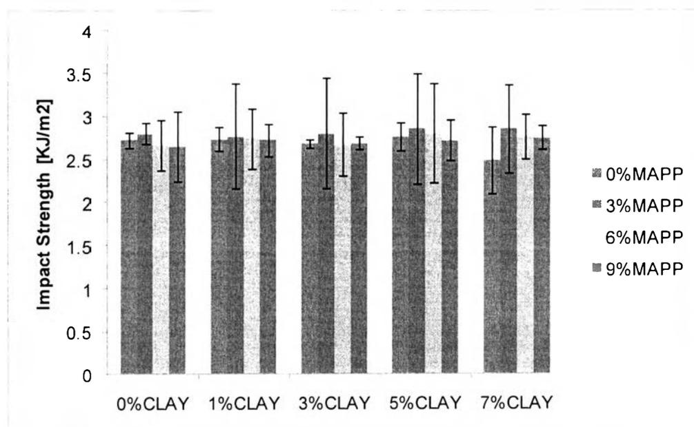
**Figure 4.4** Impact strength of WPC at nanoclay content of 0%, 1%, 3%, 5% and 7% w/w at different MAPP levels.
