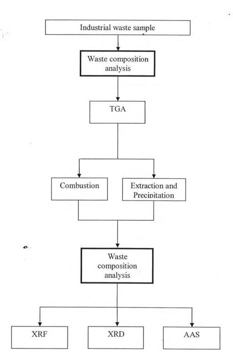
Figure 3.2 Process flow diagram of experiment.
