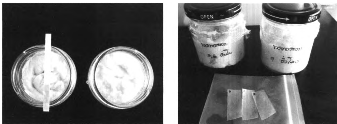
Figure 7.2 Setup for ammonia sensing (fish spoilage) by mangosteen-dyed EVA films.
