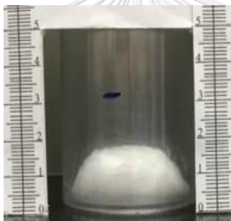
Figure 11 Determination apparatus of the relatively change in volume reduction and height of saccharide fiber.
