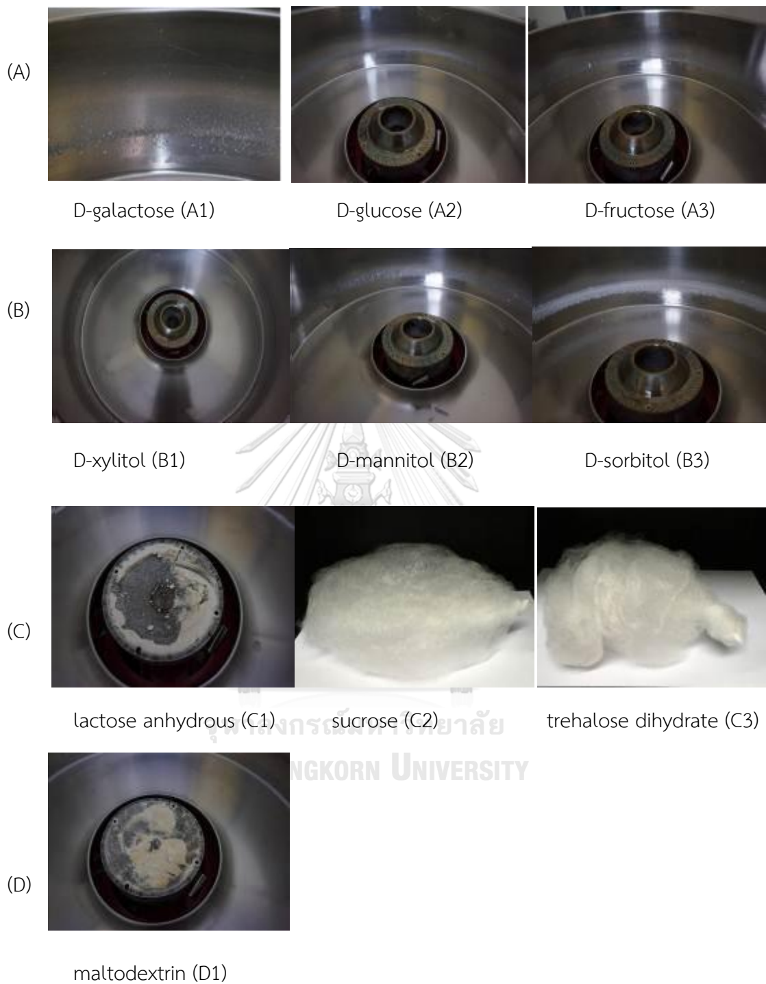
Figure 13 Physical appearance of saccharide fiber produced from different saccharide groups. (A) monosaccharide (B) sugar alcohol (C) disaccharide and (D) polysaccharide
