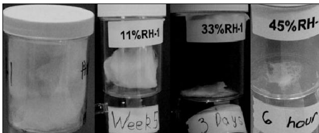
Figure 3 The physical appearance of sucrose derived cotton candy produced by centrifugal spinning under different storage conditions (33)
