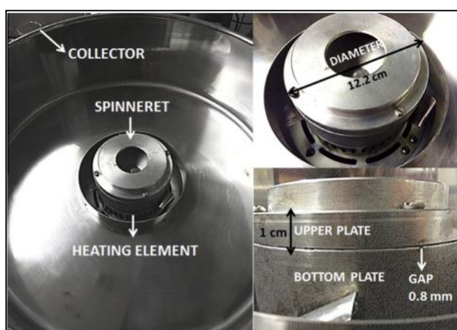
Figure 2 Compartmental of centrifugal spinning equipment (4)
