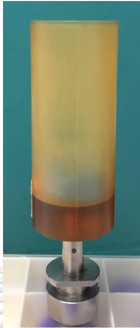
Figure 3 The specimen in sample holder for MicroCT scanning
