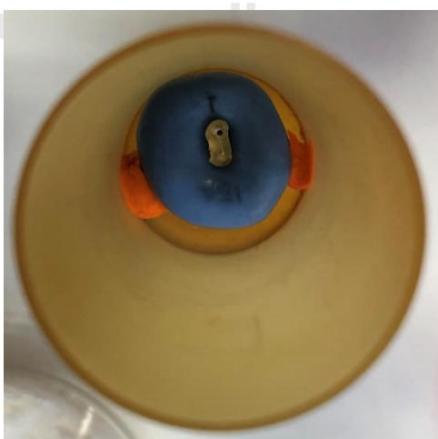
Figure 2 The specimen was mounted in silicon putty jig and fixed in the sample holder.
