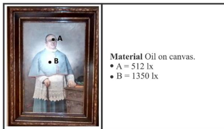
Fig. 8 - Measuring points and illuminance values over object in exhibition 4
