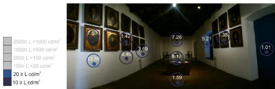
Fig. 5 - Points and values of luminance measured in scene N°10 in the 1st museum
