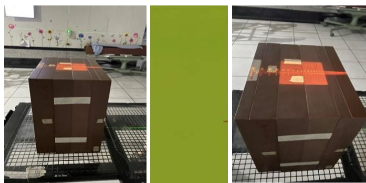
Figure 3. 16 EBT3 set-up for dose measurement.
