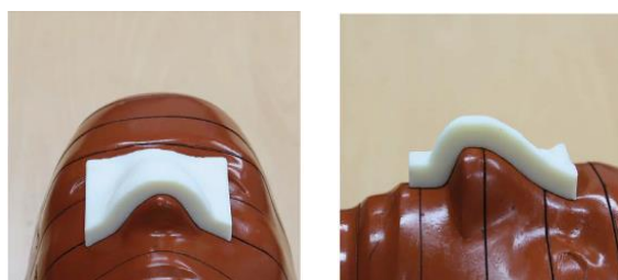
Figure 2.5: The 3D printed customized bolus on the surface of the RANDO phantom
