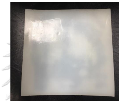
Figure 3.22: Flat customized bolus with size of 30 \times 30 \times 1 \text{ cm}^3
