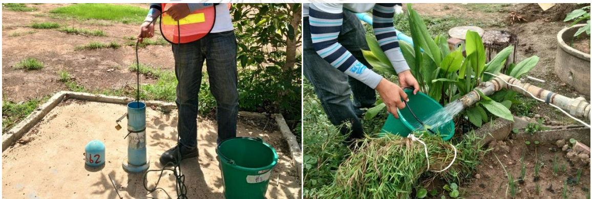
Figure 4.1 Groundwater sampling wells of the mining area (static wells; left), and the residential area (pumping wells; right)
