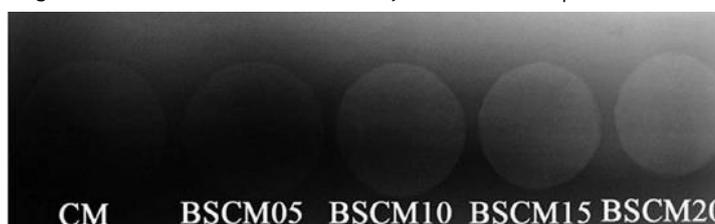
**Figure 2.14** The X-ray images of specimens under 50 kV when combining BaSO<sub>4</sub> at concentration of 0% (CM), 5% (BSCM05), 10% (BSCM10), 15% (BSCM15), and 20% (BSCM20).
