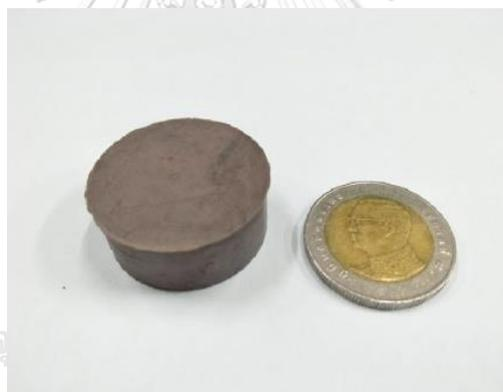
**Figure 2.15** The natural rubber combined with metal oxide for radiation shielding.
