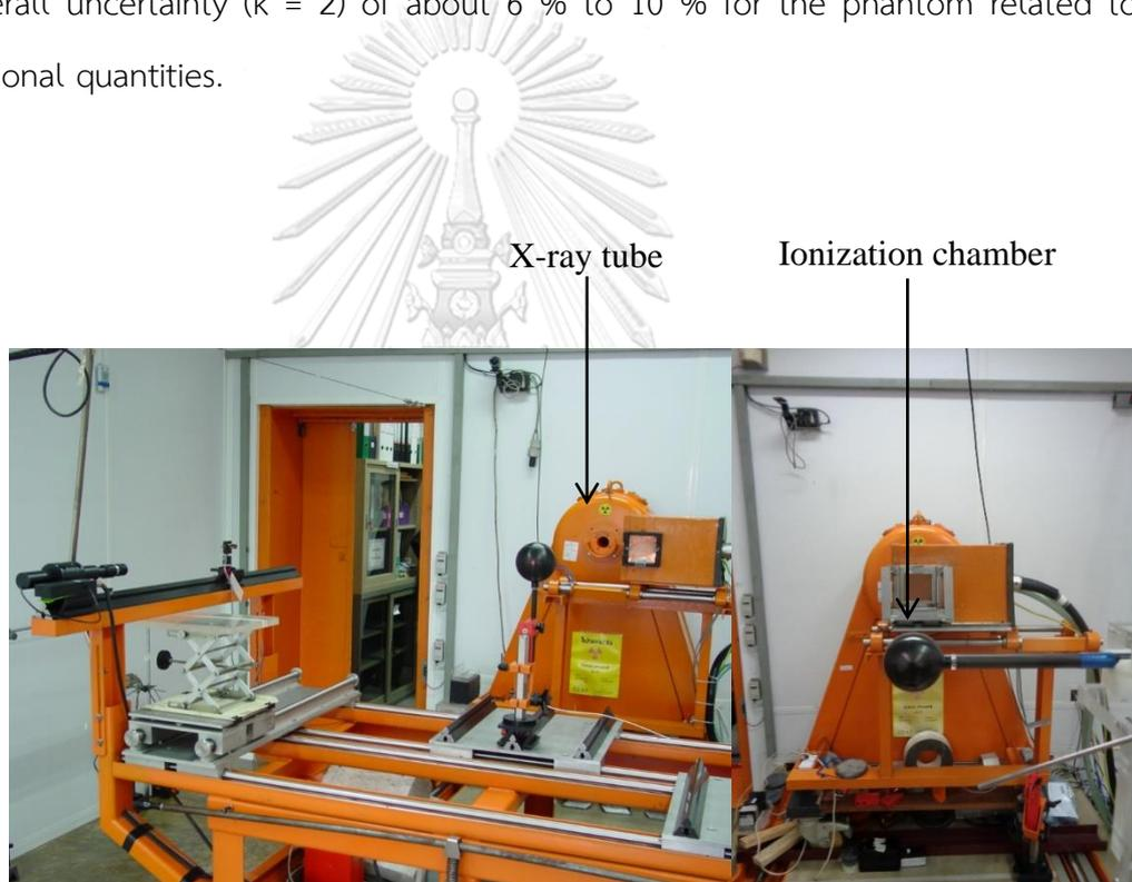
**Figure S1** X-ray calibration facilities in terms of the physical quantity air kerma.
