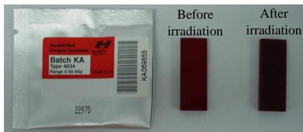
Figure S2 Red 4034 Harwell dosimeters before and after radiation.
