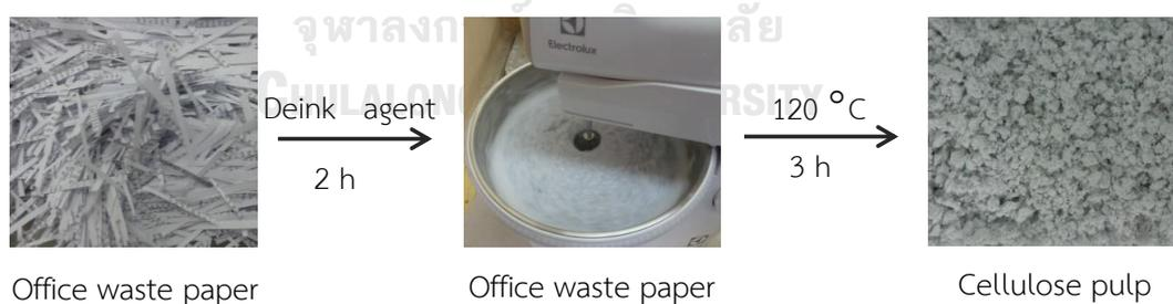
**Figure 3.1** Defiber and deink of cellulose pulp from office waste papers.
