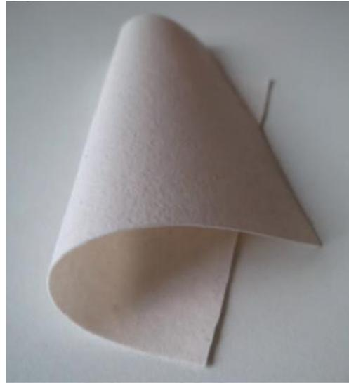
**Figure 2.11** The  $\text{BaSO}_4$  mixed with silicone rubber and coated on the cotton fabric to use as X-ray shielding aspects.
