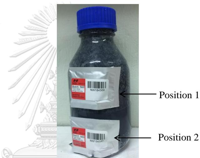
Figure S3 Red 4034 Harwell dosimeters positioned for quality control of radiation dosimetry.
