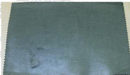
**Figure 2.13** The manufactured fiber for radiation dose reduction.
