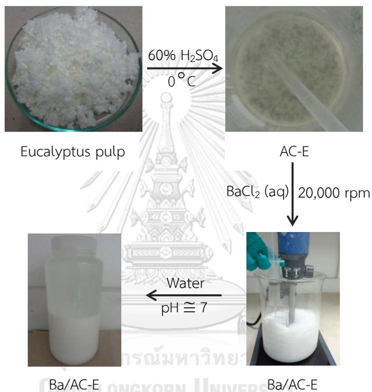
**Figure 3.4** Fabrication of Ba/AC from eucalyptus pulp.
