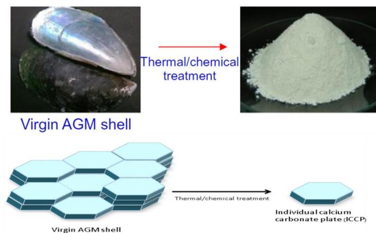
**Figure 1.3** Disintegration of stacked calcium carbonate plate into individual calcium carbonate plates
