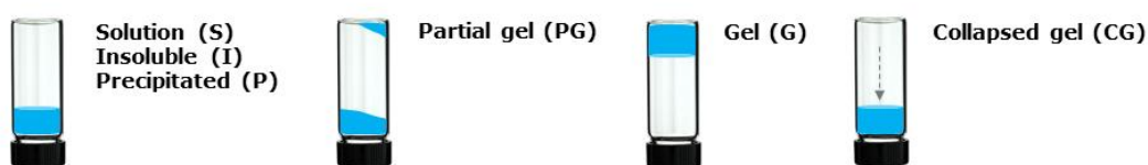
Figure 3.16 The assigned behavior of solution (S), insoluble (I), rapid precipitate formed from solution (P), partial gel (PG), gel (G) and collapsed gel (CG).
